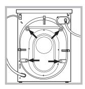
2. Remove the 4 protective screws (used during transportation) and the corresponding spacer, located on the rear part of the appliance (*see figure*).
