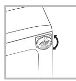
2. If the floor is uneven, the front feet of the machine may be adjusted until it reaches a horizontal position (the angle of inclination must not exceed 2 degrees). ! If the appliance is levelled correctly, it will be more stable and much less likely to cause vibrations and noise while it is operating, particularly during the spin cycle.
