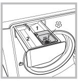
1. pre-wash compartment: use powder detergent. 2. main wash compartment: use powder or liquid detergent. If using the latter type of detergent, we recommend it is poured into the drawer immediately before you start the washing machine.
