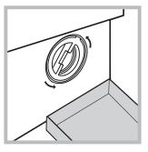
position a container so that it will collect the water which flows out (approximately 1.5 l) (see figure);
