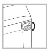
2. If the floor is uneven, the front feet of the machine may be adjusted until it reaches a horizontal position (the angle of inclination must not exceed 2 degrees). If the appliance is levelled correctly, it will be more stable and much less likely to cause vibrations and noise while it is operating, particularly during the spin cycle.
