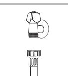
2. Connect the inlet hose by screwing it to a cold water tab using a 3/4 gas threaded connection (see figure).
