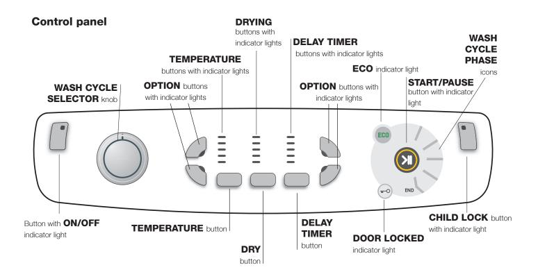
Button with () **ON/OFF** indicator light: press this briefly to switch the machine on or off. The green indicator light indicates that the machine is switched on. To switch off the washer dryer during the wash cycle, press and hold the button for approximately 3 seconds; if the button is pressed briefly or accidentally the machine will not switch off. If the machine is switched off during a wash cycle, this wash cycle will be cancelled.
