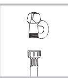
2. Connect the inlet hose by screwing it to a cold water tap using a 3/4 gas threaded connection (see figure).
