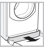
1. take off the cover panel on the front of the machine by first pressing it in the centre and then pushing downwards on both sides until you can remove it *(see figures);*
