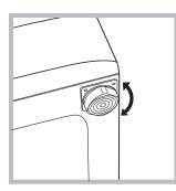
2. If the floor is uneven, the front feet of the machine may be adjusted until it reaches a horizontal position (the angle of inclination must not exceed 2 degrees). If the appliance is levelled correctly, it will be more stable and much less likely to cause vibrations and noise while it is operating, particularly during the spin cycle.If it is placed on carpet or a rug, adjust the feet in such a way as to allow a sufficient ventilation space underneath the washer dryer.
