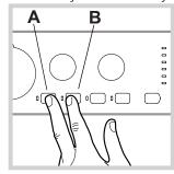
To start the programme press buttons A and **B** simultaneously for 5 seconds (see figure).
