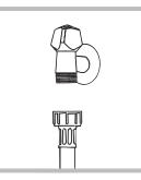
Connect the supply pipe by screwing it to a cold water tap using a 3/4 gas threaded connection (see figure).
