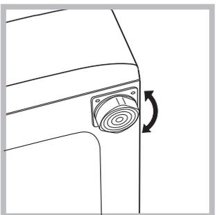
Your machine may make a considerable amount of noise if the two front feet have not been adjusted correctly.
