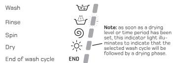
**Note:** during the "Drain" phase, the indicator light corresponding to the "Spin" cycle phase will illuminate.
