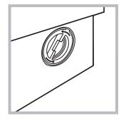
2. unscrew the lid by rotating it anticlockwise (see figure): a little water may trickle out. This is perfectly normal;
