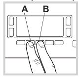
To start the programme press buttons **A** and **B** simultaneously for 5 seconds (see figure). The programme will start automatically and will run for about 70 minutes. To stop the cycle press the START/ PAUSE button.
