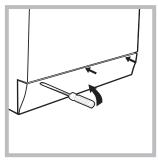
3. using a screwdriver, remove the cover panel on the lower front part of the washer-dryer (see figure).
