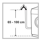
Connect the drain hose, without bending it, to a draining duct or a wall drain situated between 65 and 100 cm from the floor;
