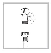
2. Connect the inlet hose by screwing it to a cold water tap using a 3/4 gas threaded connection (see figure).
