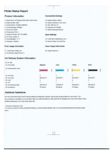
Clean the print cartridges automatically, if the diagnostic page shows steaks or missing portions of the color and black boxes.
