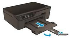
b. Slide paper-width guides outward.Slide paper-width guide outward.
