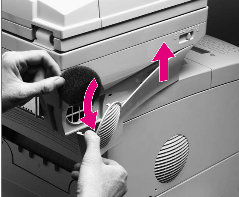
Figure 51. Remove the scan-unit left-side cover
