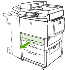
Figure 6-10 Load undetectable standard-size paper in trays 2, 3, and 4 (1 of 6)
