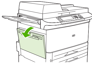
Figure 12-3 Clear jams in the duplex printing accessory (2 of 6)
