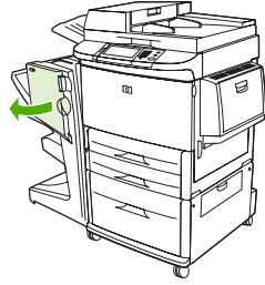
Figure 12-41 Clear a staple jam from the multifunction finisher (1 of 11)
