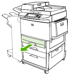
Figure 6-4 Load trays 2, 3, and 4 (1 of 6)
