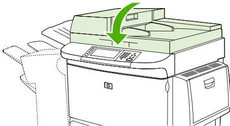
Figure 11-19 Clean the ADF rollers (3 of 6)
