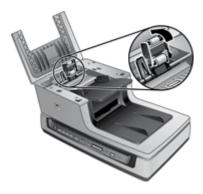
4. Inspect the separation pad that is located below the feed roller for wear and damage.
