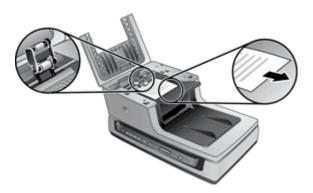
**4.** Lower the green lever to return the feed roller to the working position, and then close the ADF hatch. Press down firmly on both sides until you hear a click.
