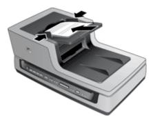
2. Adjust the paper guides to center the original. Make sure the paper guides touch the edges of the original.
