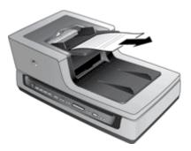
3. If the jammed page still cannot be removed, lift the lid to its fully open position, loosen the jammed page from the roller on the underside of the lid, and then gently pull the page out of the ADF.
