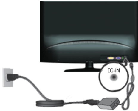
Figure 3-4 Connecting the power cable
