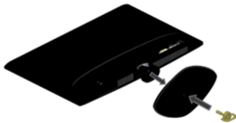
Figure 3-1 Installing the Base
