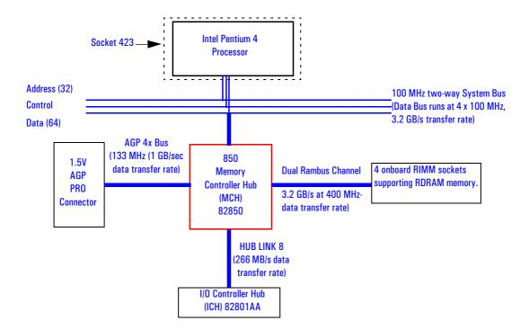
The supported operating frequency of the GTL+ bus for the Pentium 4 is 100 MHz. The width of the data bus is 64 bits, while the width of the address is 32 bits. Data bus transfers occur at four times the system bus, at 400 MHz. Along with the operating frequencies, the processor voltage is set automatically.
