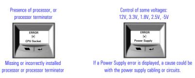
The following diagram shows how the Pre-boot Diagnostics works when it encounters an error.
