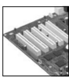
There is a total of five Peripheral Component Interconnect (PCI) 32-bit, 33 MHz connectors on the system board.
