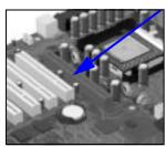
Minitower models of the HP Kayak XU700 are equipped with a single AGP (Accelerated Graphics Port) graphics slot.
