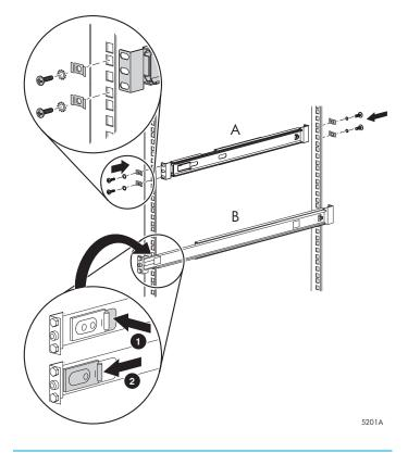
**IMPORTANT:** For hardware-mounted rails, HP recommends leaving the screws loose until the server is completely installed. This eases installation by preventing binding of the server in the rack.
