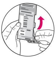
**b** Remove the bottom tab and the backing from the overlay.
