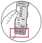
**a** Bend the bottom of the control panel overlay.
