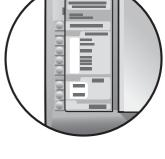
**d** Press down on the overlay to ensure it is firmly attached. Do not press on the LCD area. The tabs must be in the slots.
