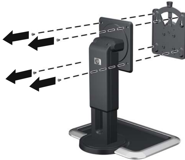
Figure 3-12 Removing the HP Quick Release from the Pedestal Base
