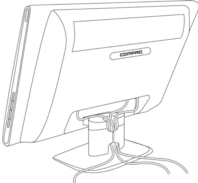
Figure 3-12 Routing cables through the rear of the support column
