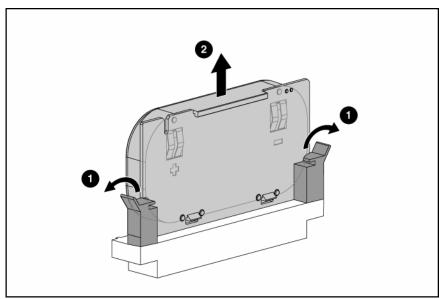
Press the battery retainer tabs down, and push them through to the other side of the cache board (1).
