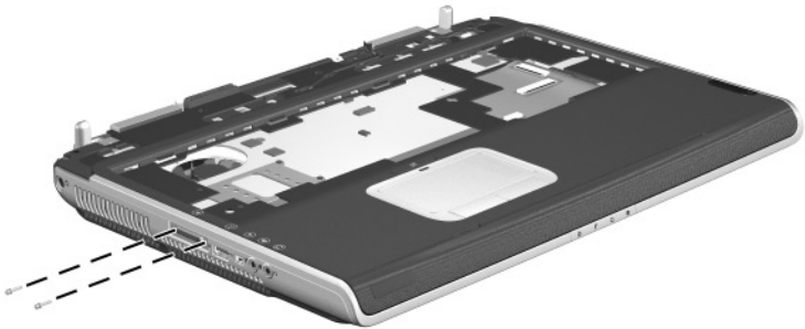
Slotted M1.5×10.0 Shoulder Screw Locations
