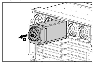
**2.** Position the fan so that the LED is near the interconnect bay, and slide the fan into the enclosure until it locks into place.
