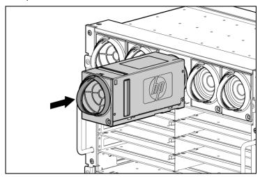
To remove a fan, turn the fan handle counterclockwise, and pull the fan from the enclosure.
