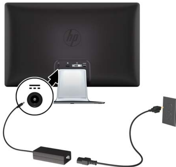
Figure 3-6 Connecting the Power Cord
