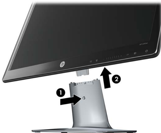
Figure 2-1 Removing the Monitor Panel
