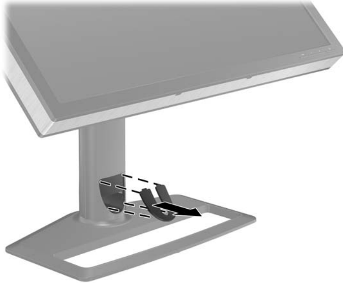
Figure 3-3 Removing the Cable Routing Cover
