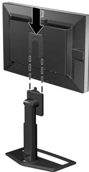
Figure 3-1 Inserting the Monitor into the Pedestal Base
