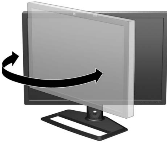
Figure 3-8 Swiveling the Monitor
