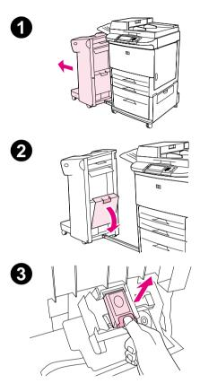
Insert the new staple cartridge, and push down on the green tab so that the cartridge locks into place.
