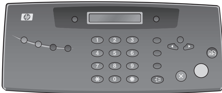
Figure 2-4 Control panel of HP 1040 Fax
