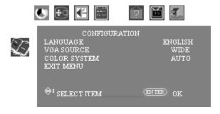
**3** Highlight and select Color System so it turns red. Adjust the setting so it reads Auto, NTSC, or PAL, and then press Setting front panel button (Enter on the remote control).
