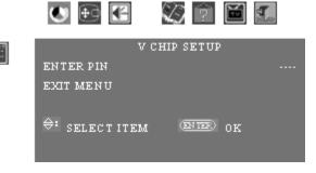
5 Highlight and select Enter Pin so it turns red, use the remote control number buttons to enter the pin (the TV comes with pin 0000 until you change it), and then press Enter on the remote control. The expanded V Chip Setup screen appears.
