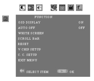
4 Highlight V Chip Setup, and then press Enter on the remote control. The V Chip Setup screen appears.
