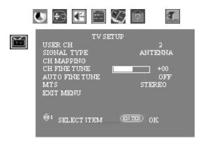
4 Highlight and select Signal Type so it turns red. Adjust the setting so it is correct for your set up (Antenna or Cable), and then press Setting front panel button (Enter on the remote control).
