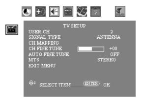
**4** Highlight and select User CH so it turns red. Adjust the setting so it reads the channel number you want to fine tune, and then press Setting front panel button (Enter on the remote control).
