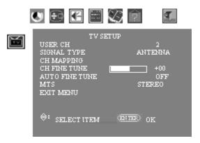
**4** On the TV Setup menu, select CH Mapping, and then press Setting front panel button (Enter on the remote control). The Channel Mapping menu appears.
