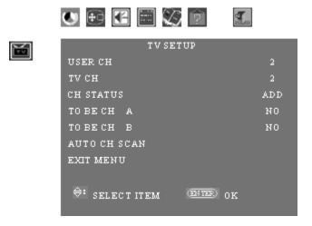
**5** Highlight and select User CH so it turns red. Adjust the setting so it reads the channel number you want to make a favorite, and then press Setting front panel button (Enter on the remote control).
