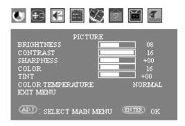
To display a menu, highlight the menu and then press the button to execute it. The text of the current highlighted item in the submenu displays in green. The text displays in red when selected for adjustment. Adjust the setting and then press the execute button to accept it. Choose Exit Menu to exit the menu, and then select the Exit menu icon or press Menu to close the display. The menu disappears after 20 seconds of no operation.
