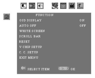
**4** Highlight C.C. Setup, and then press Setting front panel button (Enter on the remote control). The C.C. Setup screen appears.
