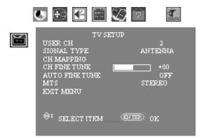
**4** On the TV Setup menu, select CH Mapping, and then press Setting front panel button (Enter on the remote control). The Channel Mapping menu appears.
