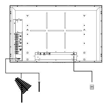
Use standard 75-ohm coaxial cable to connect a ground antenna or cable TV signal cable to the TV. Use shielded coaxial cable to reduce radio frequency (RF) interference. To make this connection:
