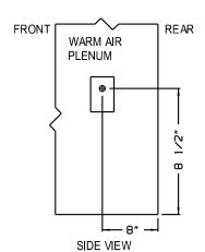
1. Using sheet metal screws, attach the damper motor in the lower right corner of the cabinet front panel as shown below. Note: The mounting holes are pre-drilled at the factory.
