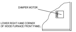
2. Attach the damper chain to the hole on the immediate left of the bottom hole in the motor wheel as shown below.
