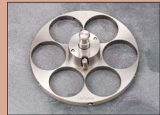
60-2100 Single Force Specimen Holder Plate, With Six 2" (50mm) Cavities. Use distance rings for smaller size specimens.
