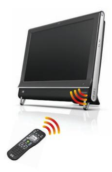
The remote control works with Windows Media Center and other software. This remote control helps you navigate on the computer just as a TV remote control helps you navigate cable TV options or control the playback of a movie in a DVD player.
