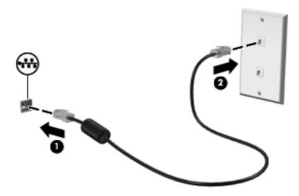
NARNING! To reduce the risk of electric shock, fire, or damage to the equipment, do not plug a modem cable or telephone cable into an RJ-45 (network) jack.
