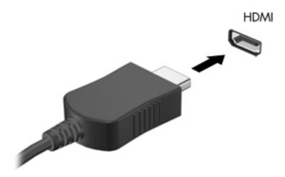
Connect the other end of the cable to the video device, and then refer to the device manufacturer's instructions for additional information.
