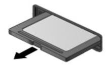
NOTE: If the card does not eject, pull the card out of the slot.
