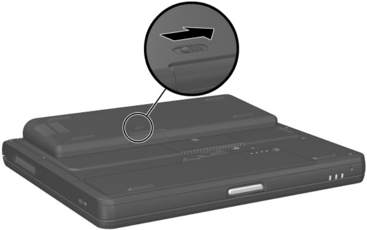
Locking the optional travel battery caddy onto the notebook
