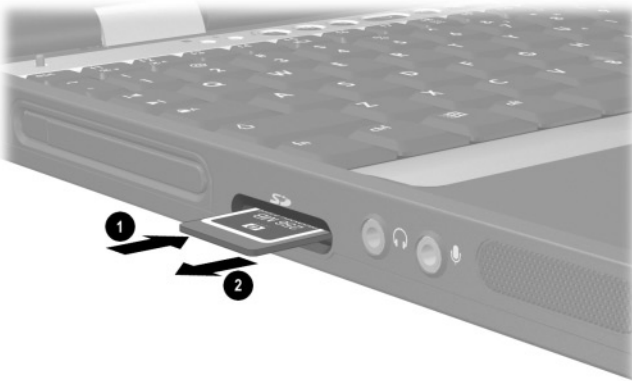
Ejecting an SD Card from the SD slot
