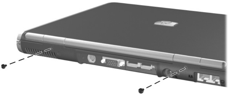
Removing the Display Assembly Screws
