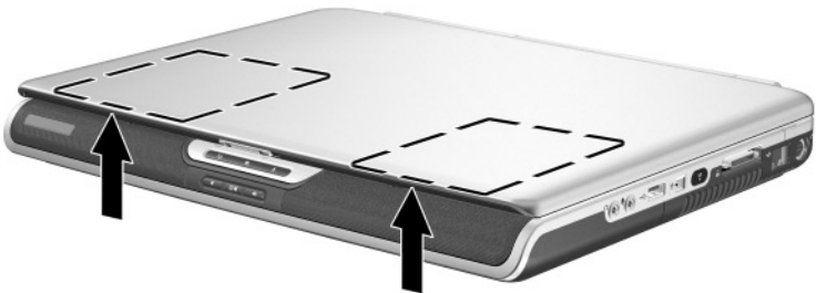
Identifying the wireless antenna
