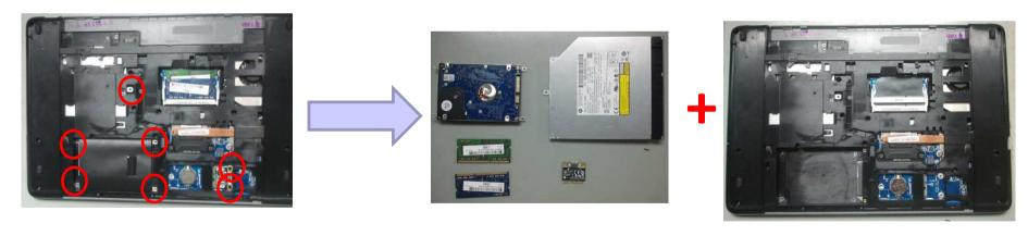
Loose HDD & ODD module screws and take off HDD & ODD module from system.
