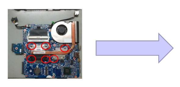
Loose screw of thermal module from MB, take off thermal module
