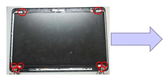
Loose LCD & Hinge screw, take off LCD, hinge and panel.
