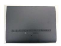
Take off the battery package from system bottom side. Release DIMM/HDD door knob and take off DIMM/HDD door.
