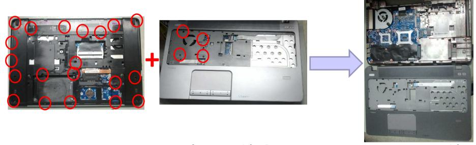
Loose L-case to U-case screws on bottom side & U-case to L-case screw on top side, and take off U-case from system. **Wistron**
