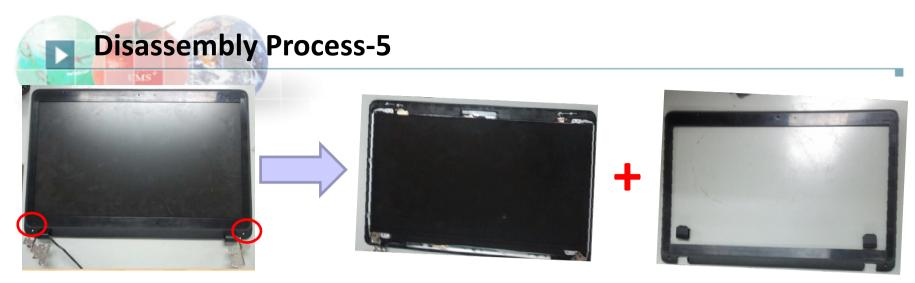
Loose screw and screw mylar, take off hinge cover and lcd bezel.
