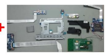
Loose the screw of the speaker ,power board, function board, touchpad module,
