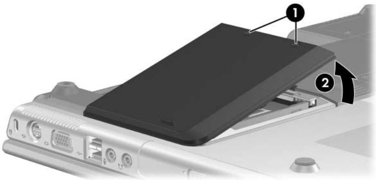
Removing the Hard Drive Cover
