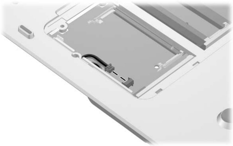
Disconnecting the Speaker Cable
