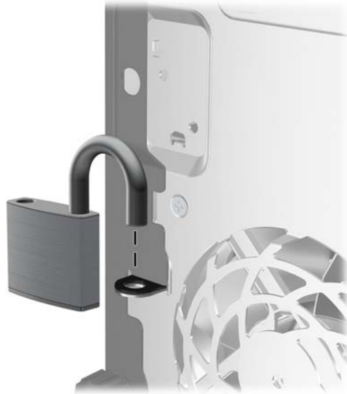
Figure C-2 Installing a Padlock
