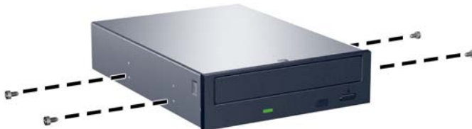
Figure 2-23 Installing Guide Screws (Optical Drive Shown)
