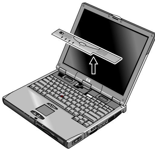
Figure 2-9. Removing the Power Button Panel
