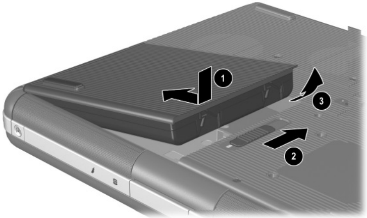
Inserting or removing the battery pack
