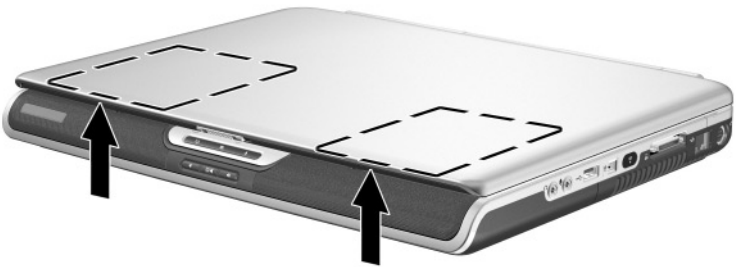
Identifying the wireless antenna
