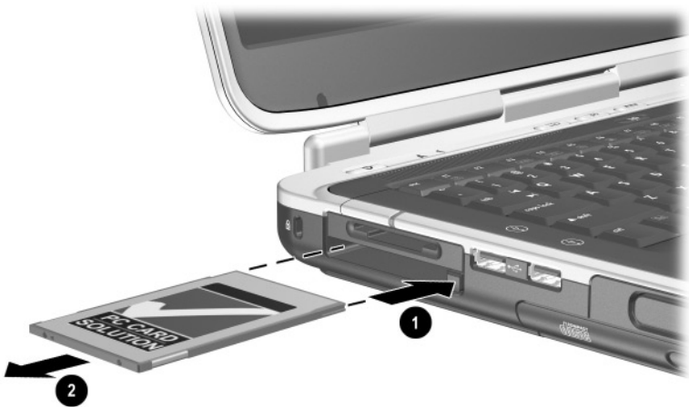
Removing a PC Card
