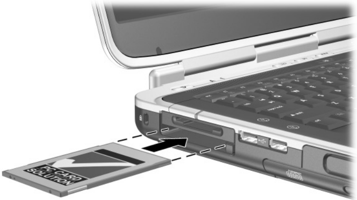
Inserting a PC Card
