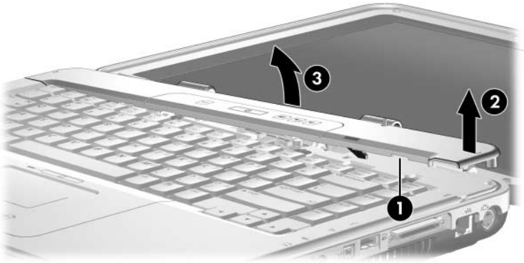
Releasing the Keyboard Cover, Compaq Presario R4000 Models
