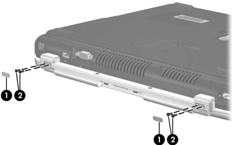
Removing the Display Screws, HP Pavilion zv6000 Models
