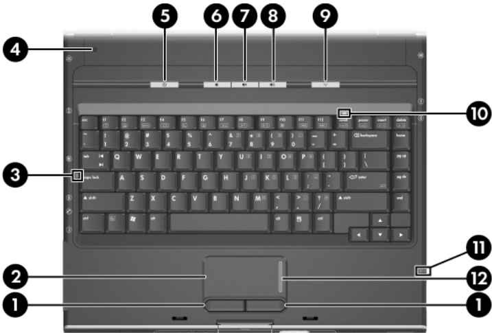
Top Components, HP Pavilion ze2000
