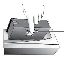
Gently press on the clip underneath the interface pod and pull the interface pod out of the analyzer.
