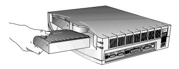
**3** Push the interface pod firmly into the analyzer until the connector at the rear is properly seated. The clip on the base of the interface pod clicks into place when the interface pod is fully inserted.
