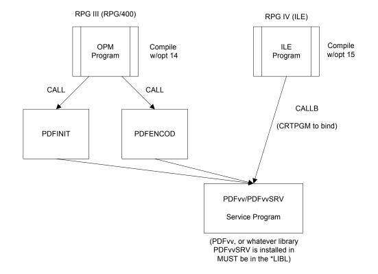
Following is a pictorial diagram of how the pieces fit together using RPG:
