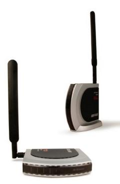
The WHR-HP-AG108's external antenna will usually give the best performance if oriented to point straight up. If your AirStation is resting on its side, use the antenna's swivel and twist function to orient it pointed upward.
