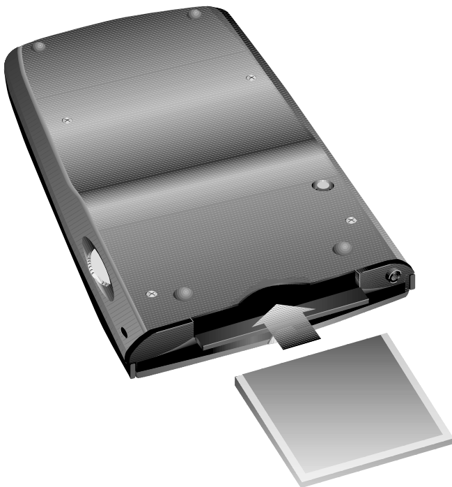
The Type I CompactFlash card slot.
