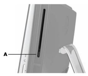
To eject a disc, make sure the power is turned on and then press the Eject button (**A**) on the side of the disc drive. You can also tap the **Start** button, tap **Computer**, press and hold (or with the mouse, right-click) the CD drive, and then tap **Eject**.
